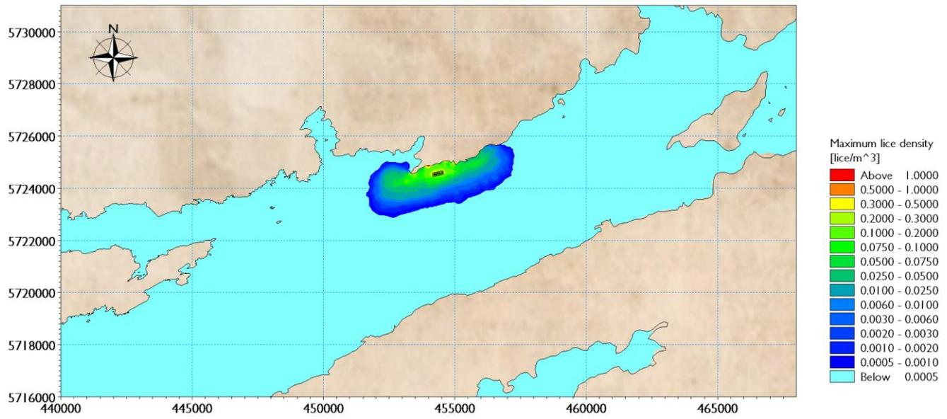
**Figure 5.41: Maximum Plume Envelope, copepodid population from 1 ovigerous louse/fish for the Shot Head site only, non-susceptible period**
