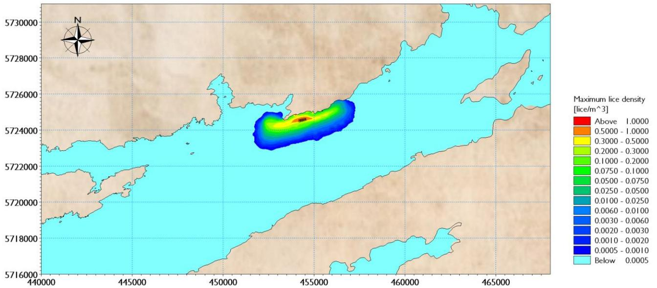
**Figure 5.43: Maximum Plume Envelope, total population (i.e. Nauplii + Copepodids) from 1 ovigerous louse/fish for the Shot Head site only, non-susceptible period**
