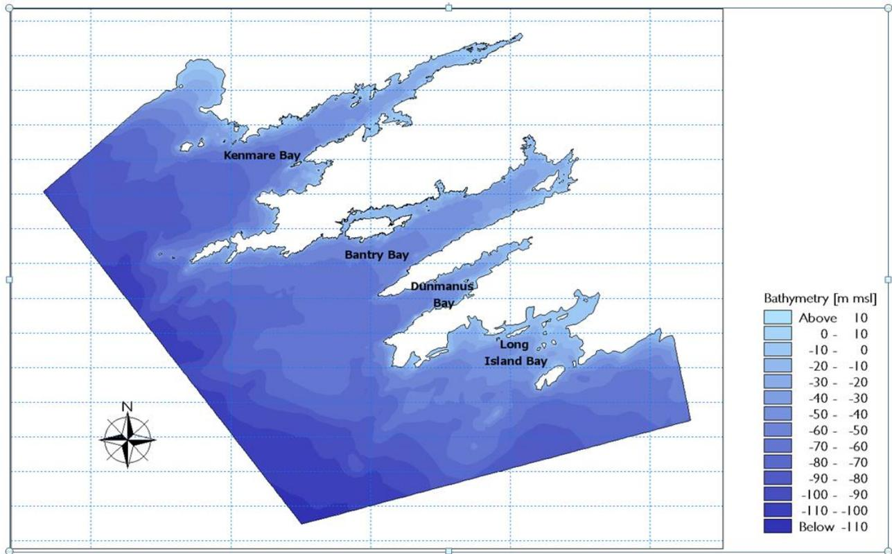
Figure 3.5: Extent of tidal model bathymetry (MSL)
